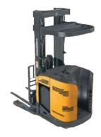
Doubledeep racks are serviced by specialized double deep reach trucks that have a pantograph that allows the forks to travel further into the racks to reach the second pallet.
