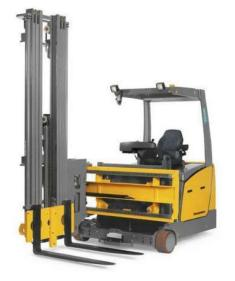
The man down swing reach turret truck is similar to the man up model but the operator remains at ground level at all times. More suitable for warehouses where the racks are 20 ft. or less, this model still features the 180°mast swing, along with the reach functionality.
